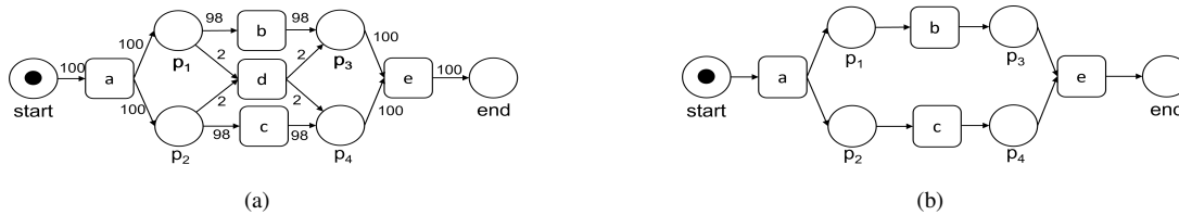
Figure 7. Petri nets for L = [(a, b, c, e)^{45}, (a, c, b, e)^{53}, (a, d, e)^2] (a) A model with frequencies, and (b) a reduced model with a 5% filter. Places are labeled start, p_1, p_2, p_3, p_4, end .
